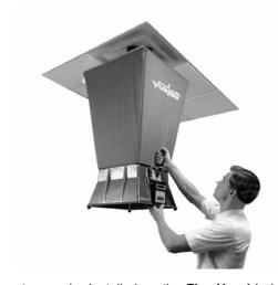
This meter can be installed on the **FlowHood** in less than 60 seconds. Airflow readings are automatically corrected for air density and backpressure at supply or exhaust outlets.
